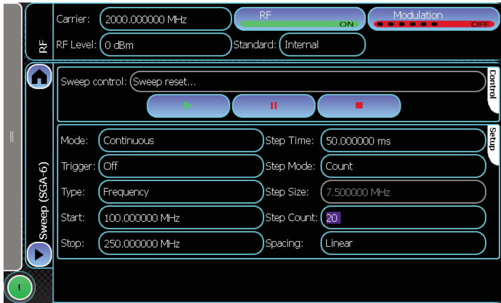
Typical frequency sweep set-up
